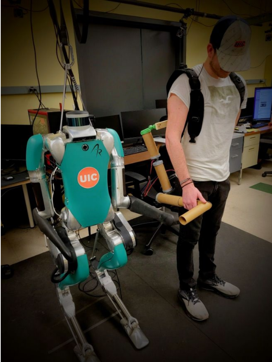
Figure 7: Finalized design of tele-operated mechanical arm control modeled next to UIC Robotics and Motion Laboratory bi-pedal robot.
